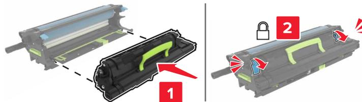
**8** Insert the imaging unit.
