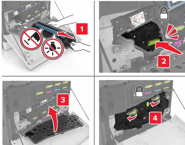
**9** Insert the waste toner bottle.
