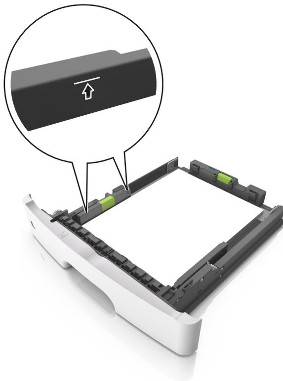
**6** Insert the tray.
