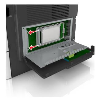
**c** Tighten the two screws.
