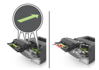
7 Insert the toner cartridge into the printer by aligning the side rails of the cartridge with the arrows on the side rails inside the printer.
