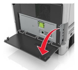
**2** Open the controller board shield using the green handle.
