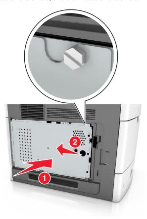
Tighten the screws on the shield.
