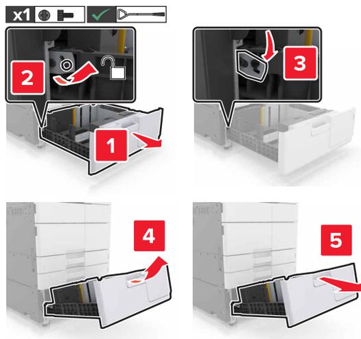
**3** Open door C. Make sure that it does not hit any cable attached to the printer.
