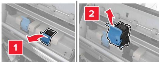
**3** Remove the empty staple cartridge from the cartridge holder.
