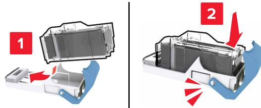
**5** Push the cartridge holder into the finisher until the holder *clicks* into place.
