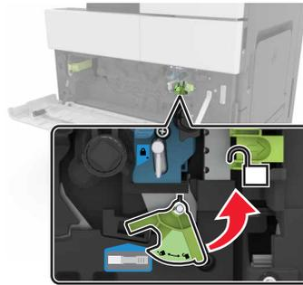
4 Remove the photoconductor unit.
