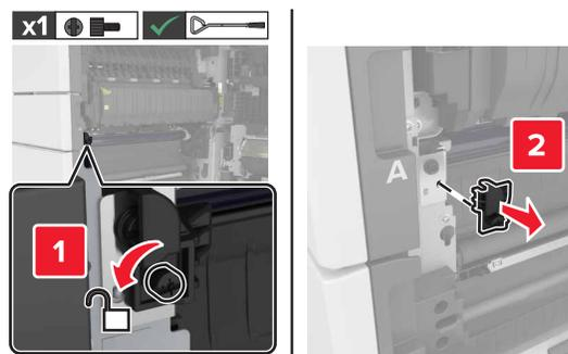
4 Loosen the screws of the transfer module lock.
