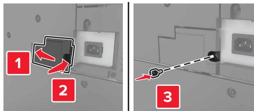
**12** Connect the power cord to the printer and electrical outlet.
