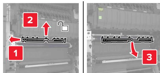
6 Lift the transfer module using the handles, and then pull it out completely.
