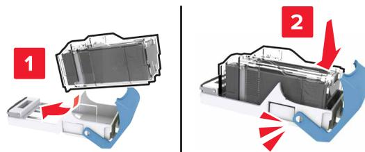
**5** Push the cartridge holder into the finisher until the holder *clicks* into place.
