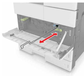
**5** Remove the printhead wiper.
