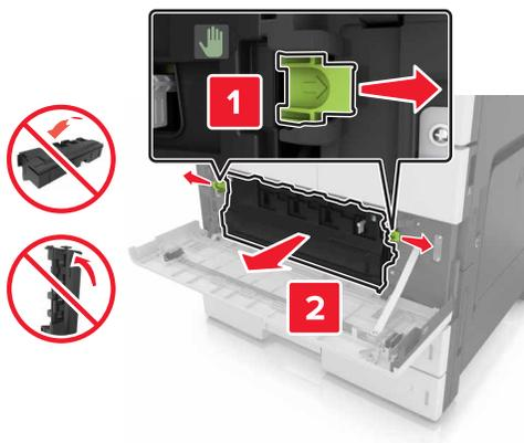
3 Unlock the photoconductor unit.
