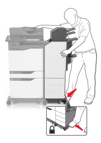
**15** Give the finisher a hard pull to check if it detaches from the printer. If the finisher detaches, then repeat step 13 and step 14 until they are properly locked.
