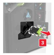
**3** Open the staple guard, and then remove the loose staples.
