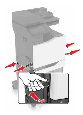
**Note:** If optional trays are already installed, then unlock them from the printer before lifting the printer. Do not try to lift the printer and trays at the same time.
