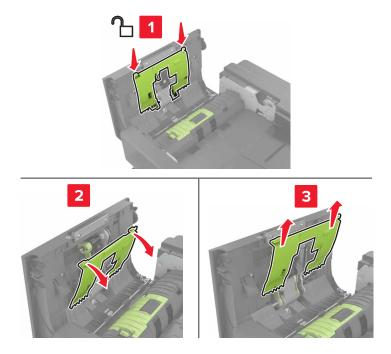
4 Remove the ADF feed roller.
