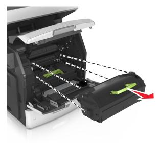
**3** Lift the green handle, and then pull out the imaging unit from the printer.
