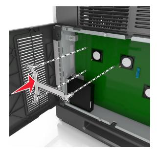
**Note:** Make sure that the plastic bracket has latched completely, and that the plastic bracket is seated firmly on the cage.
