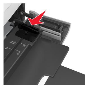
Note: Use the paper size indicators on the bottom of the tray to help position the guides.
