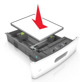
• If you are loading envelopes, then make sure that the flap side is facing up and the envelopes are on the left side of the tray.
