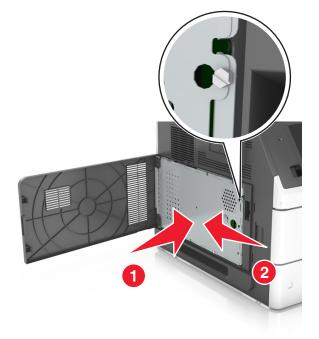
**6** Tighten the screws on the shield.
