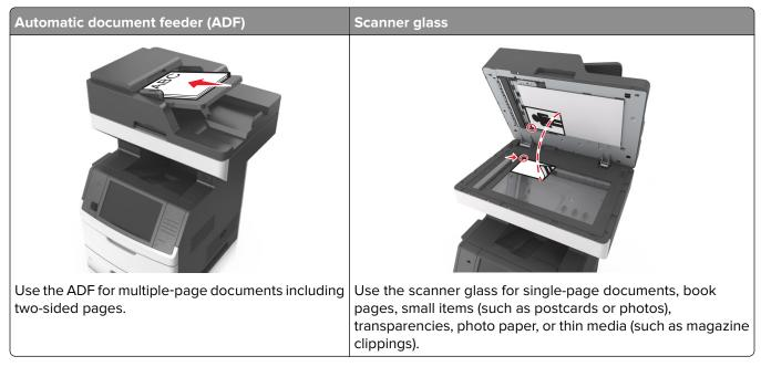
The scanner lets you scan documents directly to a computer or a flash drive. The computer does not have to be directly connected to the printer for you to receive images using Scan to Computer. You can scan the document back to the computer over the network by creating a scan profile on the computer and then downloading the profile to the printer.
