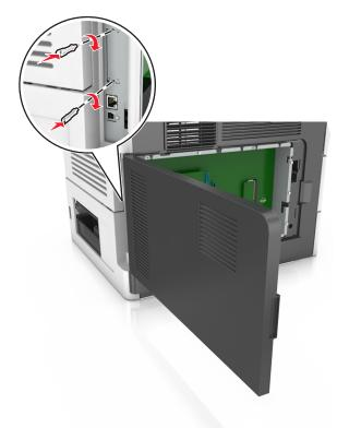
10 Tighten the thumbscrew that is attached to the ISP.Warning—Potential Damage: Do not screw it on too tightly.
