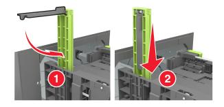
**d** Squeeze, and then slide the length guide to the correct position for the paper size you are loading.
