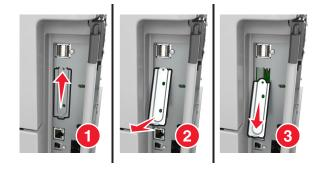
**5** Align the posts of the plastic bracket to the holes on the controller board cage, and then press the plastic bracket on the controller board cage until it *clicks* into place.
