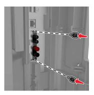
6 Remove the thumbscrews that attach the hard disk mounting bracket to the hard disk, and then remove the bracket.
