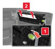
**4** Open the standard trays, and then locate the jammed paper.
