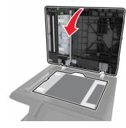
**6** Push the corners of the ADF scan pad to secure it into place.
