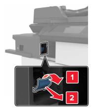
**3** Remove the empty staple cartridge from the cartridge holder.
