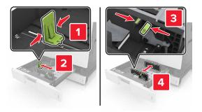
Note: Use the indicators on the bottom of the tray to position the guides.
