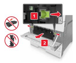
**3** Unlock the photoconductor unit.
