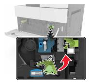
**4** Remove the photoconductor unit.
