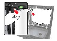
**3** Unpack the new ADF scan pad, and then remove the packing materials.
