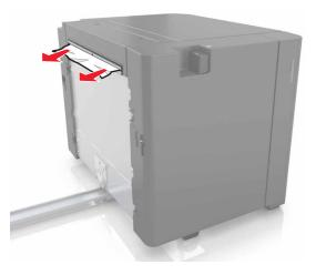
3 Open door F, and then remove the jammed paper.Note: Make sure that all paper fragments are removed.
