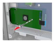
**5** Secure the ISP mounting bracket to the controller board cage using the screws.
