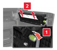
**3** Open the standard trays, and then locate the jammed paper.
