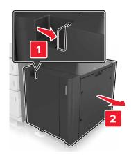
**2** Open door C. Make sure that it does not hit any cable attached to the printer.
