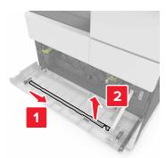
6 Insert the wiper into the hole until it stops, and then slide it out. Repeat three times.
