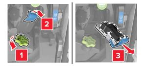
**3** Remove the empty staple cartridge from the cartridge holder.
