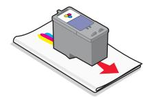
**4** Using another clean section of the cloth, gently hold the cloth against the contacts for about three seconds, and then wipe in the direction shown.
