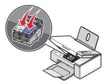
**5** Lift the scanner unit, gently push the scanner support towards the cartridge carriers, and carefully lower the scanner unit until it is completely closed.
