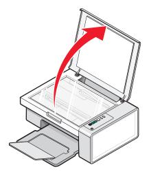
**6** Place the printed alignment page facedown on the scanner glass in the lower right corner, and then close the top cover.
