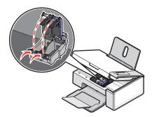
**3** Insert the black cartridge or the photo cartridge in the left carrier. Insert the color cartridge in the right carrier.
