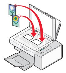
**Note:** For best results, place photos with the most space possible between photos and the edges of the scan area.
