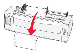
**11** Place the paper holes over the tractor pins.
