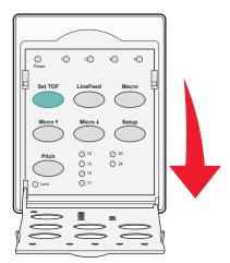
**6** Press any paper movement button (**LineFeed**, **Micro** ↑, **Micro** ↓) to align the horizontal lines located on the platen with the Top-Of-Form you want.
