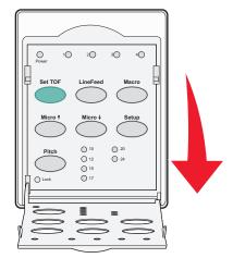
**5** Press any paper movement button (**Micro** ↑, **Micro** ↓, **LineFeed**) to align the horizontal lines located on the platen with the Top-Of-Form you want.
