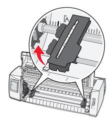
**7** Open the left and right tractor doors, and then place the paper holes over the second or third pins of the tractor unit.
