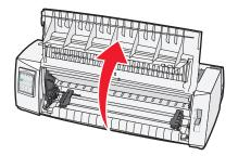
Hold down the latching levers while you lift and pull the tractor unit out of the printer.
