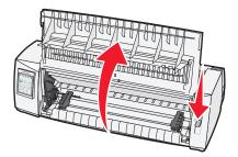
While holding down the latching levers, fit the left and right locks onto the posts in the printer.
