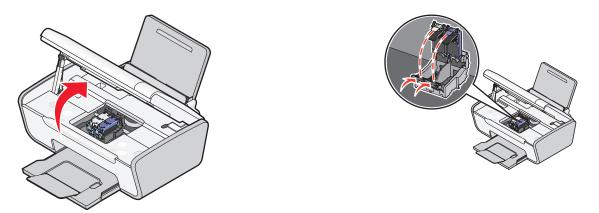
7 Remove the tape from the black cartridge, insert the cartridge in the left carrier, and then close the black cartridge carrier lid.
