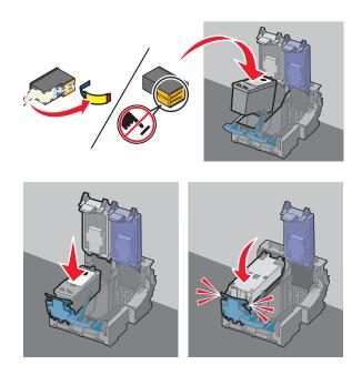
8 Remove the tape from the color cartridge, insert the cartridge in the right carrier, and then close the color cartridge carrier lid.
