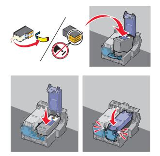
**Warning—Potential Damage:** Do *not* touch the gold contact area on the back or the metal nozzles on the bottom of the cartridge.
