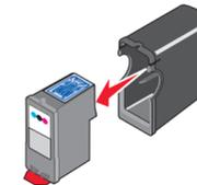
**2** Remove the sticker and tape from the print cartridges.
