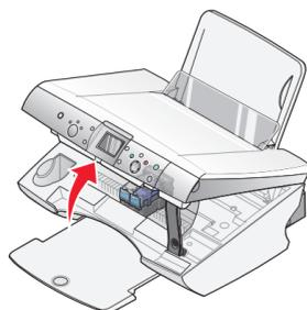
**2** Open the cartridge lids, insert the cartridges, and snap the lids closed.
