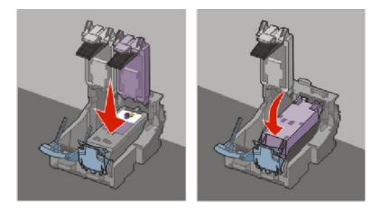
**Warning—Potential Damage:** Do *not* touch the gold contact area on the back or the metal nozzles on the bottom of the cartridge.
