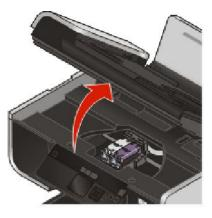
**3** Press down on the cartridge carrier latch to raise the cartridge carrier lid.
