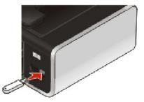
Note: An adapter may be necessary if your flash drive does not fit directly into the port.
