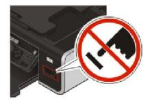
**Note:** The printer recognizes one active media device at a time. If you insert more than one media device, a message appears on the display prompting you to designate the device you want the printer to recognize.
