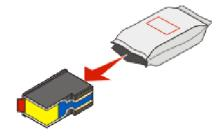
**14** If a storage unit is included, remove the color cartridge from the storage unit.
