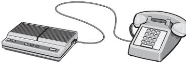
5 Connect a third telephone cord from the answering machine to the EXT port
