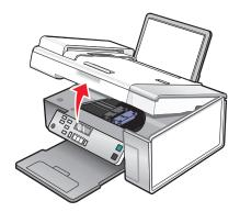
**3** Press down on the cartridge carrier lever to raise the cartridge carrier lid.
