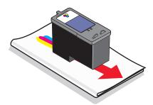
**4** Using another clean section of the cloth, gently hold the cloth against the contacts for about three seconds, and then wipe in the direction shown.
