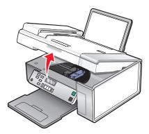
Press down on the print cartridge carrier levers.
