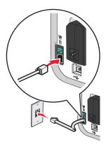
**3** Remove the protective plug from the EXT port  $\widehat{\blacksquare}$  of the printer.
