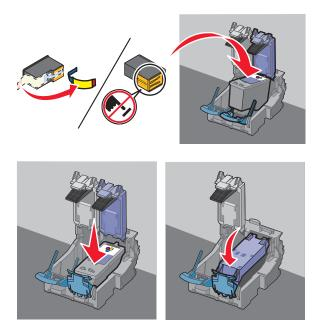
**19** If a black print cartridge is included in the box contents, open the black cartridge foil, and then remove the cartridge from the pack.
