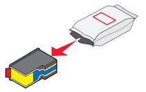
17 If a storage unit is included, remove the color cartridge from the storage unit.
