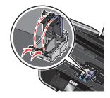
**18** Open the color cartridge foil, and then remove the cartridge from the pack.
