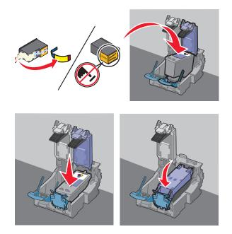
If a black print cartridge is included in the box contents, open the black cartridge foil, and then remove the cartridge from the pack.
