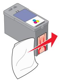
**5** With another clean section of the cloth, repeat step 3 and step 4, and then let the nozzles and contacts dry completely.
