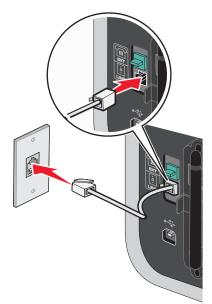
**3** Remove the protective plug from the EXT port  $\stackrel{\frown}{\boxplus}$  of the printer.
