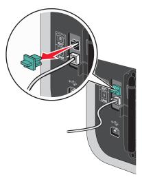
**4** Connect a second telephone cord from the computer modem to the EXT port 🗐 of the printer.
