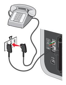
5 If you would like to use the same line for recording messages on your answering machine, connect a second telephone line (not provided) between the answering machine and the other N slot of the telephone wall jack.
