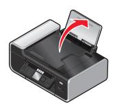
4 If a correct control panel for your language needs to be installed, open the printer and raise the control panel.
