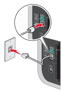
**3** Remove the protective plug from the EXT port m of the printer.
