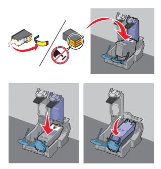
**21** If a black print cartridge is included in the box contents, open the black cartridge foil, and then remove the cartridge from the pack.
