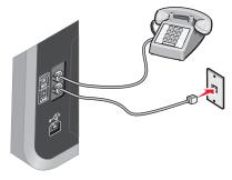
**Warning—Potential Damage:** Do not touch cables or the printer in the area shown while actively sending or receiving a fax.
