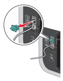
**4** Connect the other telephone cord to a telephone, and then plug it into the EXT port  $\widehat{\ }$  of the printer.
