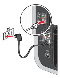
**4** If you would like to use the same line for both fax and telephone communication, connect a second telephone line (not provided) between the telephone and the F slot of an active telephone wall jack.
