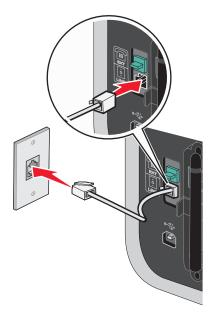
**3** Remove the protective plug from the EXT port  $\widehat{\ }$  of the printer.
