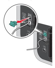
**4** Connect a second telephone cord from the computer modem to the EXT port  $\widehat{\ }$  of the printer.
