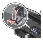
**18** Open the color cartridge foil, and then remove the cartridge from the pack.
