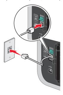
**3** Remove the protective plug from the EXT port of the printer.
