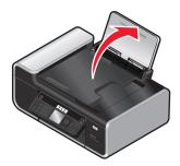
4 If a correct control panel for your language needs to be installed, open the printer and raise the control panel.
