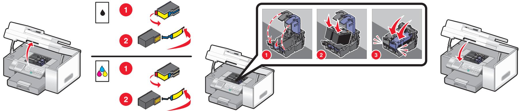
**7** The printer automatically aligns the print cartridges and prints an alignment page. This may take a few minutes.
