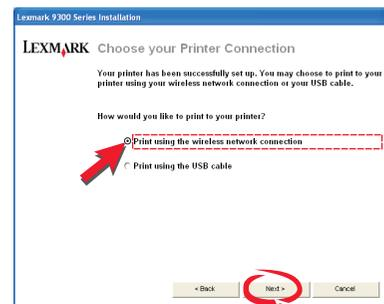
**20** When configuration is complete, disconnect the Wireless Network Configuration cable, and then click **Next**.
