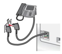
5 If you would like to use the same line for recording messages on your answering machine, connect a second telephone line (not provided) between the answering machine and the other N slot of the telephone wall jack.
