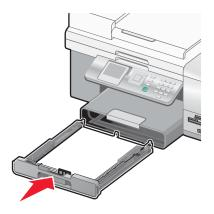
**Note:** The tray cannot be completely inserted so it is flush with the printer front if you extended the tray to accommodate A4- or legal-size paper. Do not try to force the tray in further.
