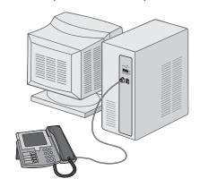
**5** Connect a third telephone cord from the computer modem to the EXT port  $\stackrel{\text{(iii)}}{=}$  of the printer.
