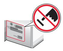
**Note:** The printer recognizes one active media device at a time. If you insert more than one media device, a message appears on the display prompting you to designate the device you want the printer to recognize.
