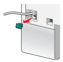
**4** Connect the other telephone cord to a telephone, and then plug it into the EXT port  $\stackrel{\frown}{\boxplus}$  of the printer.
