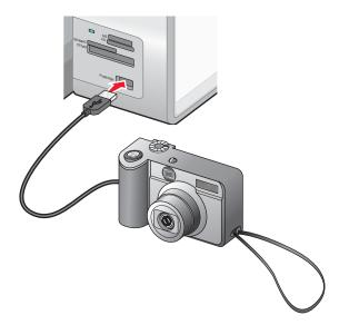
**Warning:** Do not touch the USB cable, any network adapter, or the printer in the area shown while actively printing from a PictBridge-enabled digital camera. A loss of data can occur. Also, do not remove the USB cable or network adapter while actively printing from a PictBridge-enabled digital camera.
