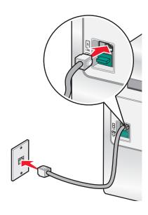
${\bf 3}\,$  Remove the protective plug from the EXT port  $\widehat{\ }$  of the printer.
