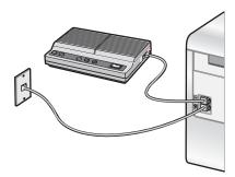
Warning: Do not touch cables or the printer in the area shown while actively sending or receiving a fax.
