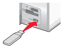
Note: An adapter may be necessary if your flash drive does not fit directly into the port.
