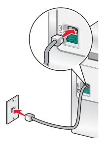
**3** Remove the protective plug from the EXT port  $\stackrel{\square}{=}$  of the printer.
