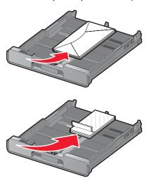
**5** Adjust the paper guides to rest gently against the left, right, and bottom edges of the envelopes or photo cards.
