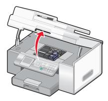
2 Grasp the control panel at the front. Lift and rotate it back to remove it (if one is installed).
