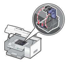
4 Insert the black cartridge or photo cartridge in the left carrier. Insert the color cartridge in the right carrier.
