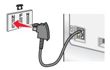
4 If you would like to use the same line for both fax and telephone communication, connect a second telephone line (not provided) between the telephone and the F slot of an active telephone wall jack.
