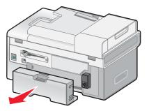
3 Push down on the button on the rear access door.
