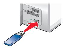
Note: A converter cable may be necessary if your Bluetooth adapter does not fit directly into the port.
