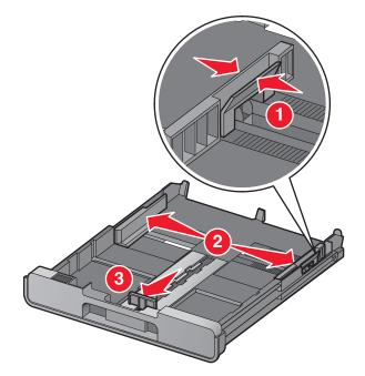
**Note:** If you are loading A4- or legal-size paper, squeeze the lever and pull to extend the tray. It is unnecessary to extend the tray for paper sizes shorter in length than A4 or legal, such as letter-size paper. When you pull the extension out, the first stop accommodates A4-size paper. When the extension is fully out, it accommodates legal-size paper.
