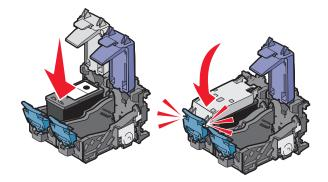
**4** Remove the tape from the back and bottom of the color cartridge, and insert the cartridge in the right carrier.
