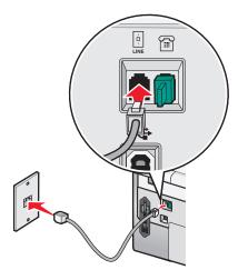
${\bf 3}~$  Remove the protective plug from the EXT port  $\widehat{\mbox{\sc in}}$  of the printer.
