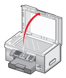
**3** Place the original document facedown on the scanner glass in the upper left corner. The arrows which surround this corner remind you of the proper placement.
