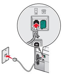
**3** Remove the protective plug from the EXT port 🗐 of the printer.
