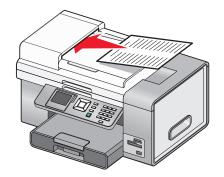
**Note:** Do not load postcards, photos, small items, or thin media (such as magazine clippings) into the Automatic Document Feeder. Place these items on the scanner glass.
