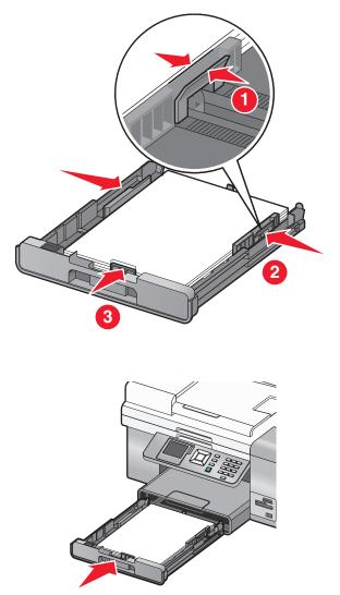
**Note:** The tray cannot be completely inserted so it is flush with the printer front if you extended the tray to accommodate A4- or legal-size paper. Do not try to force the tray in further.
