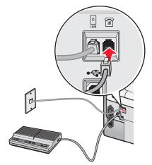
**Warning—Potential Damage:** Do not touch cables or the printer in the area shown while actively sending or receiving a fax.
