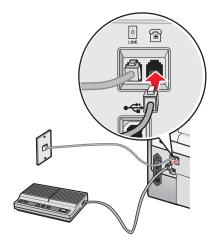
**Warning—Potential Damage:** Do not touch cables or the printer in the area shown while actively sending or receiving a fax.
