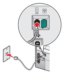
**3** Remove the protective plug from the EXT port  $\widehat{\blacksquare}$  of the printer.
