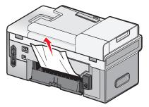
4 Push down on the duplex latch as you reinstall the duplex unit.
