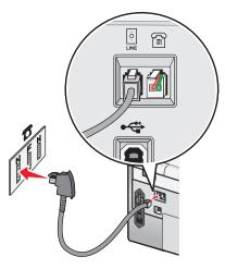
4 If you would like to use the same line for both fax and telephone communication, connect a second telephone line (not provided) between the telephone and the F slot of an active telephone wall jack.
