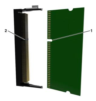
**4** Push the memory card straight into the connector, and then push the card toward the controller board wall until it *clicks* into place.
