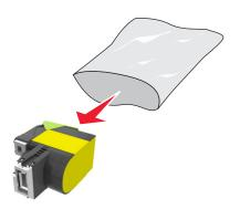
**4** Align the new toner cartridge, and then press the cartridge down until it fits into place.
