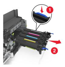
8 Remove the used developer unit.
