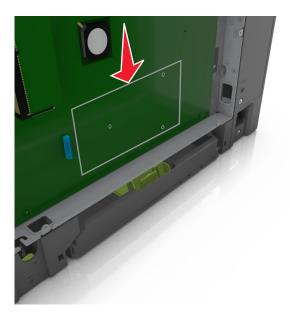
**5** Align the standoffs of the printer hard disk to the holes in the controller board, and then press the printer hard disk down until the standoffs are in place.
