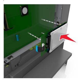
**6** Insert the plug of the printer hard disk interface cable into the receptacle of the controller board.
