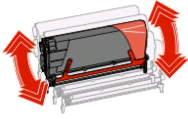
Firmly shake the toner cartridge side-to-side and front-to-back several times to distribute the toner.
