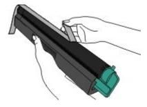
5 Insert the new cartridge into the printer and then turn the toner lock lever to the left.
