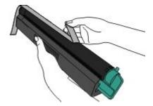
Insert the toner cartridge and turn the lock lever to the left.
