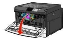
**Warning—Potential Damage:** To avoid overexposing the imaging units, do not leave the door open for more than 10 minutes.
