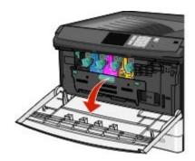
3 Push the imaging unit lock lever up and pull out the imaging unit with the toner cartridge attached to it.
