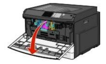
2 Turn the toner lock lever to the right and pull the toner cartridge out.
