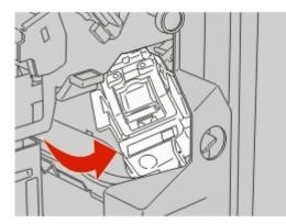
**3** Lift the lever, and then remove the staple cartridge.
