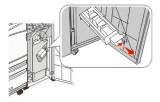
8 Remove the staple cartridge identified on the display.
