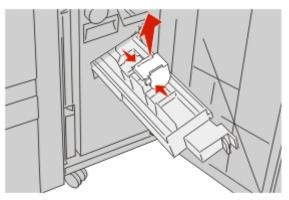
**9** Remove the jammed staples, and then place the staple cartridge into the stapler.
