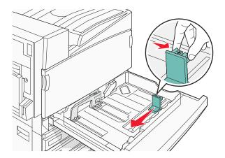
**3** Squeeze the length guide tab inward as shown, and slide the guide to the correct position for the paper size being loaded.
