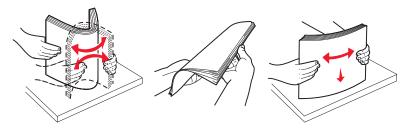
**5** Load the paper stack with the recommended print side faceup. Load the paper in either the long-edge or short-edge orientation as shown below:
