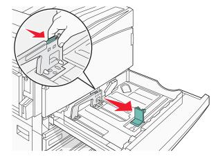
Note: Use the size indicators on the bottom of the tray to help position the guides.
