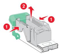
**5** Insert the front side of the new staple case into the staple cartridge, and then push the rear side into the cartridge.
