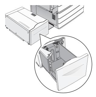
**2** Adjust the width guide as necessary.
