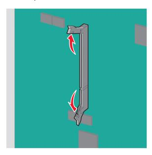
Align the notch on the memory card to the ridge on the connector.
