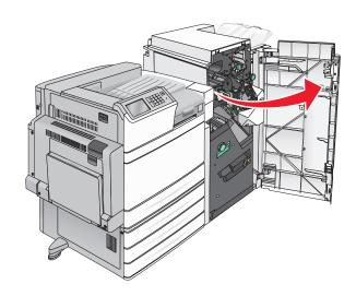
**2** Press the latch to open the stapler door.
