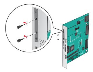
**b** Remove the screws attached to the printer hard disk mounting bracket, and then remove the bracket.
