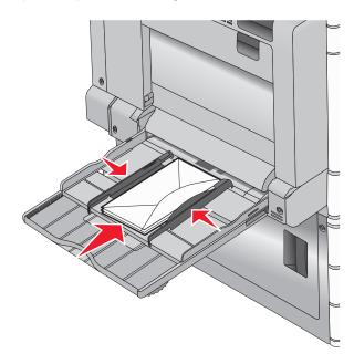
**Warning—Potential Damage:** Never use envelopes with stamps, clasps, snaps, windows, coated linings, or self-stick adhesives. These envelopes may severely damage the printer.
