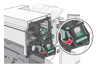
**3** Lower the latch of the staple cartridge holder, and then pull the staple cartridge holder out of the printer.
