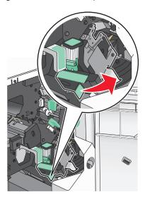
**3** Pull the staple cartridge out of the finisher.
