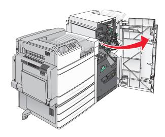
**2** Press the handles of the staple cartridge to the right, and then take the staple cartridge unit out of the finisher.
