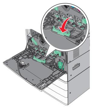
**Warning—Potential Damage:** To avoid overexposing the photoconductor unit, do not leave the door open for more than 10 minutes.
