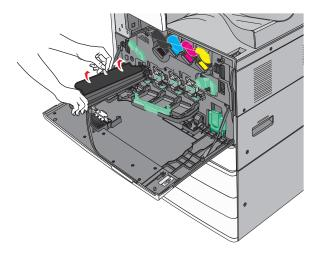
Push the tab forward to insert the photoconductor unit.
