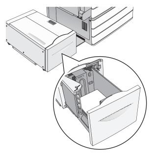
**Note:** Make sure the paper is below the maximum fill line located on the edge of the paper tray. Overloading the tray can cause paper jams and possible printer damage.
