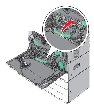
Rotate the release lever clockwise to lock the cover.
