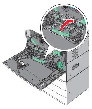
Slide the release lever to the right to lock the cover.
