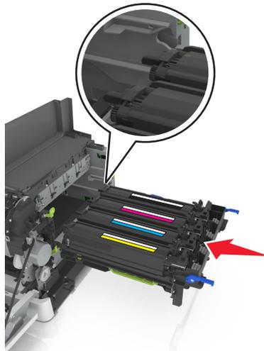
**13** Push the blue levers down until the imaging kit is fully seated into place.
