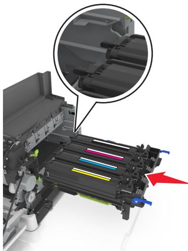
**15** Push the blue levers down until the imaging kit is fully seated into place.
