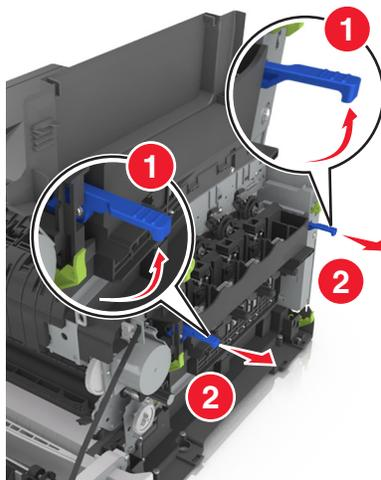
7 Press down the blue lever, and then grasp the green handles on the sides to pull out the imaging kit.
