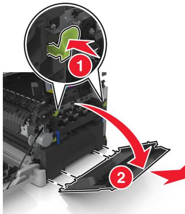
5 Press the green levers on each side of the waste toner bottle, and then remove the waste toner bottle.
