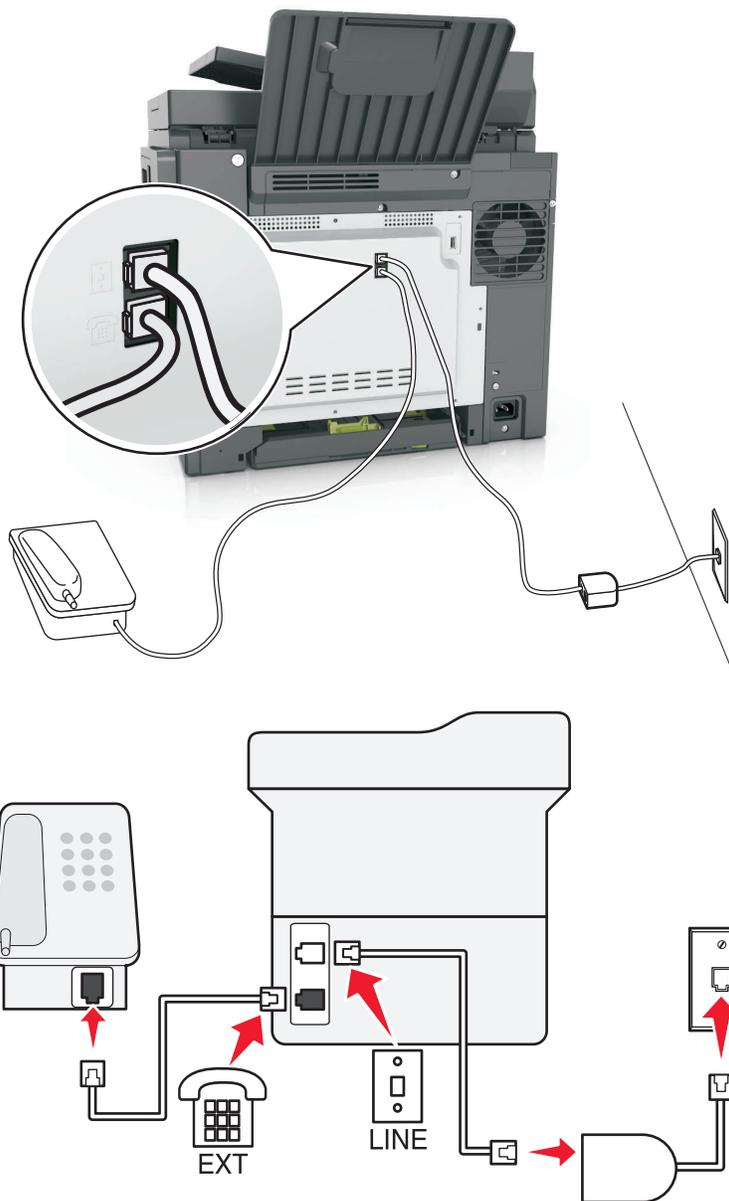
A Digital Subscriber Line splits your regular telephone line into two channels: voice and Internet. Telephone and fax signals travel through the voice channel, and Internet signals pass through the other channel. This way, you can use the same line for analog voice calls (including faxes) and digital Internet access.
