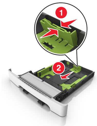
**Note:** Use the paper size indicators on the bottom of the tray to help position the guide.
