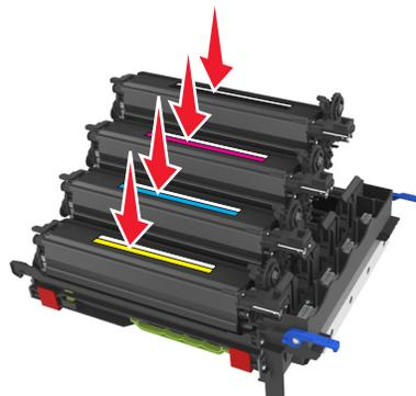
**Note:** Make sure each developer unit is inserted into the matching color slot.
