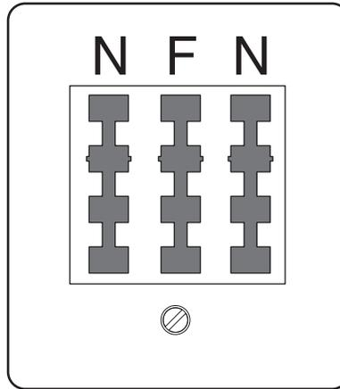
Connect the printer to any of the N ports.
