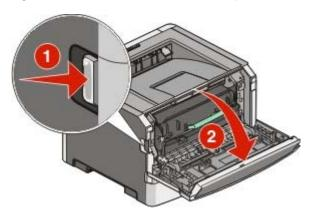
**2** Press the button on the base of the photoconductor kit, and then pull the toner cartridge out using the handle.
