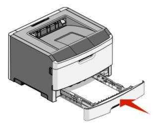
**8** If a different type of paper was loaded than the type previously loaded in the tray, change the Paper Type setting for the tray from the printer control panel. For more information, see <u>"Setting the Paper Size and Paper Type" on page 26.</u>
