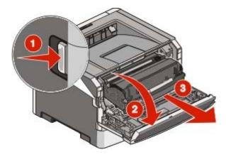
**4** Lift the flap in front of the printer, and remove any jammed sheets.
