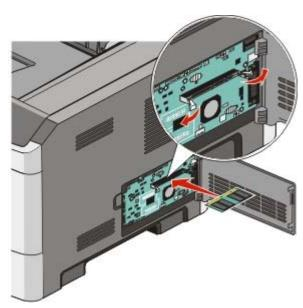
**4** Push the memory card into the connector until the latches *snap* into place.
