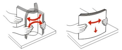
• Hold transparencies by the edges, and then fan them. Straighten the edges on a level surface.
