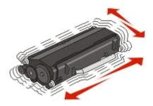
**5** Install the new toner cartridge by aligning the rollers on the toner cartridge with the arrows on the tracks of the photoconductor kit. Push the toner cartridge in as far as it will go. The cartridge *clicks* into place when correctly installed.
