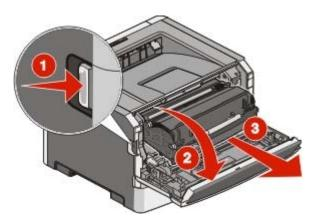
**2** Lift the flap at the front of the printer, and then remove any jammed sheets of paper that are short lengths of paper.
