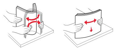
4 Load the paper stack toward the back of the tray as shown with the recommended print side facedown.
