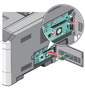
**6** Push the memory card into the connector until the latches *click* into place.
