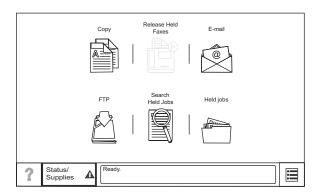
Touch on the lower right to access settings and configuration menus for the device.
