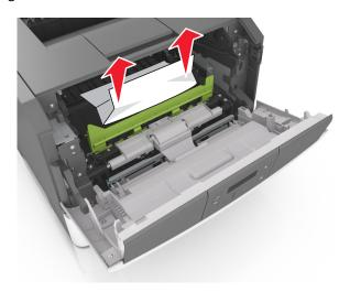
7 Insert the imaging unit by aligning the arrows on the side rails of the unit with the arrows on the side rails inside the printer, and then insert the imaging unit into the printer.
