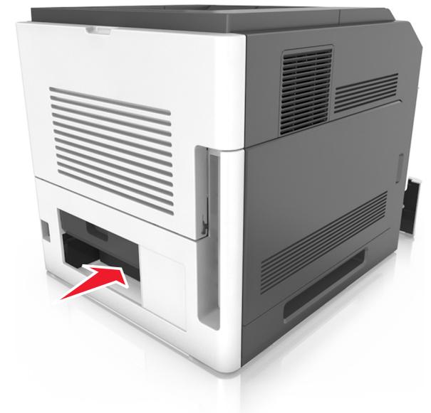
5 Press down the rear duplex flap, then firmly grasp the jammed paper, and then gently pull the paper out.
