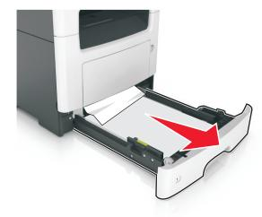
**2** Locate the blue lever, and then pull it down to release the jam.
