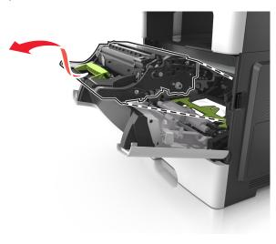
**Warning—Potential Damage:** Do not touch the shiny blue photoconductor drum under the imaging unit. Doing so may affect the quality of future print jobs.
