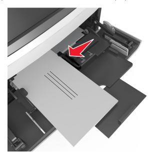
**Warning—Potential Damage:** Never use envelopes with stamps, clasps, snaps, windows, coated linings, or self-stick adhesives. These envelopes may severely damage the printer.
