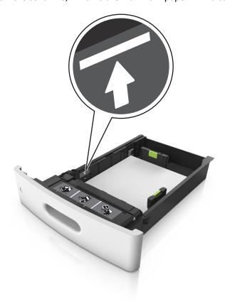
Warning—Potential Damage: Overfilling the tray can cause paper jams.
