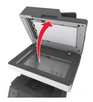
**3** Remove the white underside of the scanner cover.
