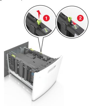
**b** Squeeze, and then slide the length guide to the position for A5 until it *clicks* into place.
