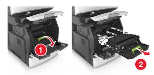
**5** Place the imaging unit aside on a flat, smooth surface.
