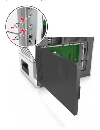
Remove the printer hard disk.
