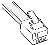
The fax ports on the back of the printer and the telephone cable that comes with the printer have RJ-11 connectors. If you have a different type of connector in your country or region, then you may need to use an RJ-11 adapter.
