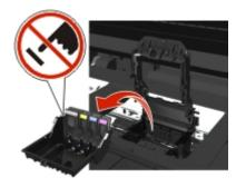
**5** Insert the supported printhead, and then close the latch until it *clicks* into place.
