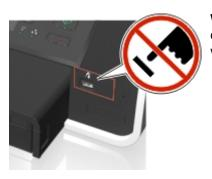
**Warning—Potential Damage:** Do not touch any open connector, the memory device, or the printer in the areas shown while actively printing, reading, or writing from the memory device. A loss of data can occur.
