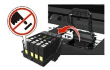
**3** Wipe the printhead contacts and the contacts inside the printhead carrier using a clean, lint-free cloth.
