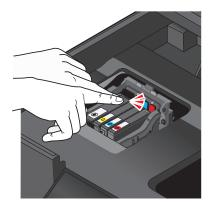
**Note:** Install the new ink cartridges immediately after removing the protective cap to avoid exposing the ink to air.
