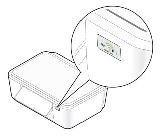
If the Wi-Fi indicator light is not lit or is orange, then try reconnecting to a wireless network.
