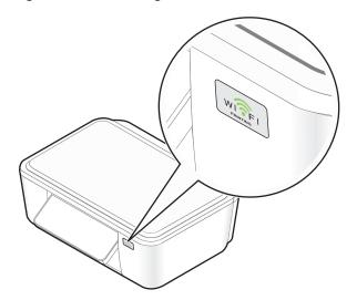
If the Wi-Fi indicator light is not lit or is orange, then try reconnecting to the wireless network.
