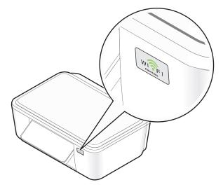
If the Wi-Fi indicator light is not lit or is orange, then run the wireless setup again.
