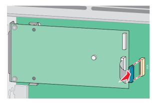
**12** If a printer hard disk was previously installed, then attach the printer hard disk to the ISP. For more information, see "Installing a printer hard disk" on page 29.
