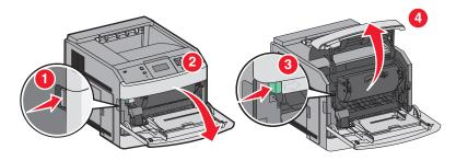
**3** Lift and pull the print cartridge out of the printer.
