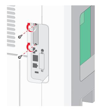
**9** Attach the two provided screws to secure the ISP mounting bracket to the system board cage.
