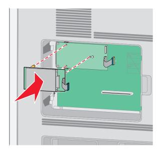
${\bf c}$   $\;$  Insert the plug of the printer hard disk interface cable into the receptacle of the ISP.
