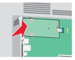
8 Insert the long thumbscrew and turn it clockwise enough to hold the ISP in place, but do not tighten the thumbscrew at this time.
