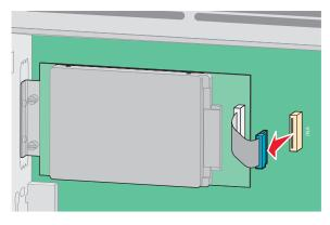
**b** Remove the screws holding the printer hard disk in place.
