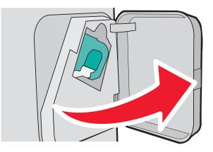
**2** Pull the latch of the staple cartridge holder down, and then pull the holder out of the printer.
