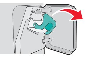
**3** Use the metal tab to lift the staple guard, and then remove any loose staples.
