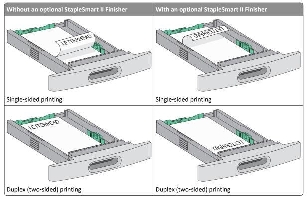
**Note:** Notice the maximum fill line on the side of the tray which indicates the maximum height for loading paper. Do not overload the tray.
