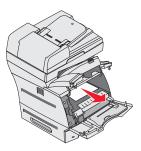
**CAUTION:** Do not use any pointed objects to remove the paper. This could cause personal injury or damage to the MFP.
