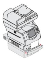
**4** Open any optional trays beginning at the top, and remove any jammed media.
