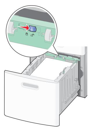
**4** Push the length guide release latch to raise the length guide, slide the guide to the correct position for the paper size being loaded, and then lock the guide.
