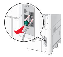
**4** Connect the other telephone cord to a telephone, and then plug it into the EXT port  $\widehat{}$  of the printer.
