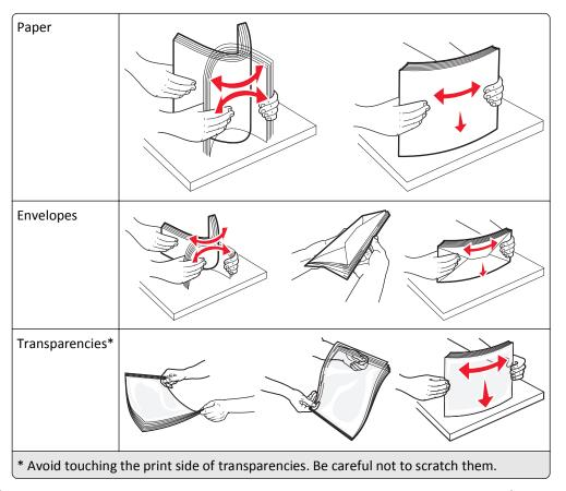
Load the paper or specialty media. Slide the stack gently into the multipurpose feeder until it comes to a stop.
