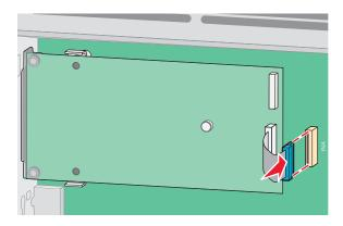
**12** If a printer hard disk was previously installed, then attach the printer hard disk to the ISP. For more information, see "Installing a printer hard disk" on page 38.
