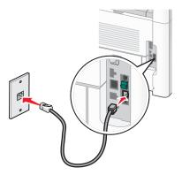
**3** Remove the protective plug from the EXT port  $\widehat{}_{||}$  of the printer.
