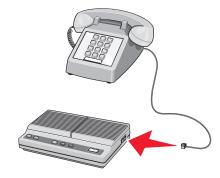
**5** Connect a third telephone cord from the answering machine to the EXT port  $\widehat{}_{||}$  of the printer.
