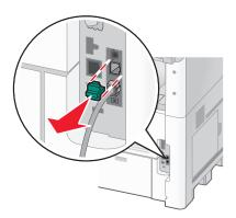
**2** Connect your telecommunications equipment directly to the EXT port  $\widehat{\ }$  on the back of the printer.
