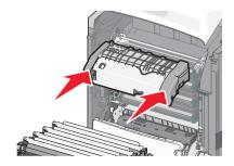
**b** Turn the screws to the right to fasten the fuser securely.
