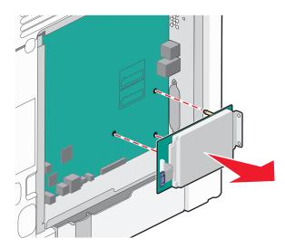
**d** Remove the thumbscrews that attach the printer hard disk mounting bracket to the printer hard disk, and then remove the bracket. Set the printer hard disk aside.
