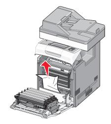
4 Pull out on the release tabs to allow the front door to split.
