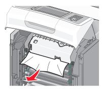
**b** If paper is not visible, then you will need to remove the fuser unit.
