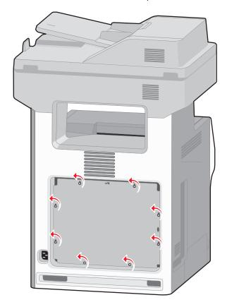
**b** Lift up on the tabs to align each screw with the corresponding keyhole.
