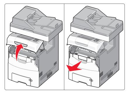
**2** Pull up and out on the green tabs of the specified cartridge to remove it from the printer.
