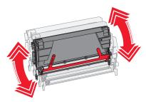
**9** Remove the red packing strips from the new cartridge.
