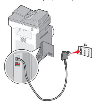
4 If you would like to use the same line for both fax and telephone communication, then connect a second telephone line (not provided) between the telephone and the F slot of an active analog telephone wall jack.
