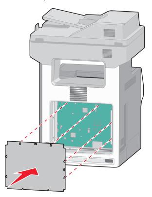
**2** Slide the cover down, and then turn each screw clockwise to tighten.
