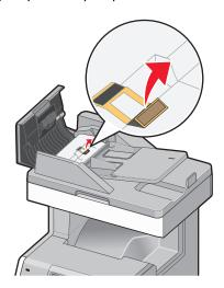
**2** Replace the pick pad with a new one, and then discard the old pad.
