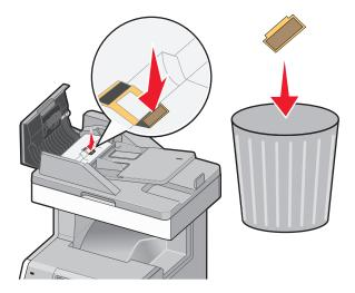
**3** Open the flap to access the sensor lens underneath, and then wipe the lens clean.
