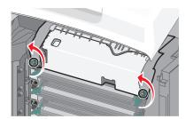
**b** Lift the handholds on each side of the fuser unit, and then pull forward to remove it.
