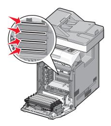
**4** Clean the lenses using a can of compressed air.
