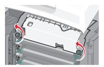
Lift the handholds on each side of the fuser, and then pull forward to remove it.
