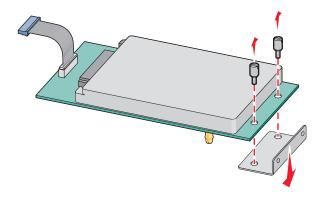
**b** Align the standoffs of the printer hard disk with the holes in the ISP, and then press downward on the printer hard disk until the standoffs have seated into place.
