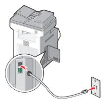
**3** Remove the plug from the printer EXT port  $\widehat{\underline{\ }}$ .
