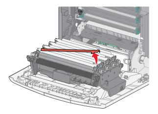
**6** Place the old photoconductor into the replacement photoconductor box, and then place the return label on the box and mail it to Lexmark for recycling.
