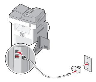
**3** Connect the answering machine or telephone to the adapter. Use one of the following methods:
