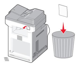
**3** Replace the air filter, and then replace the cover.
