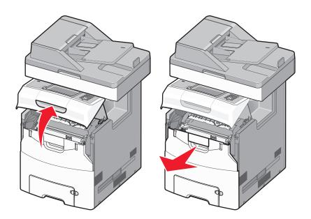
**Warning—Potential Damage:** To avoid overexposing the photoconductors, do not leave the front doors open for more than 10 minutes.
