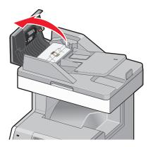
**4** Remove the pick roller assembly.
