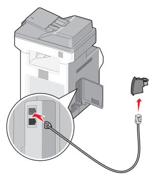
**3** Connect the adapter into the N slot of an active analog telephone wall jack.
