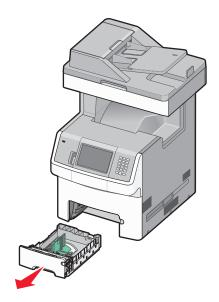
**2** Squeeze and slide the width guides to the correct position for the size of paper you are loading. Use the size indicators on the bottom of the tray to help position the guides.
