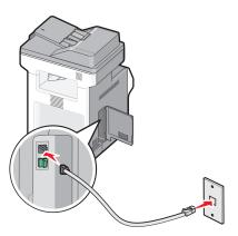
**3** Remove the protective plug from the printer EXT port  $\widehat{\mathbf{m}}$ .
