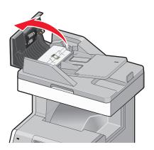
**2** Replace the pick roller assembly, as shown.
