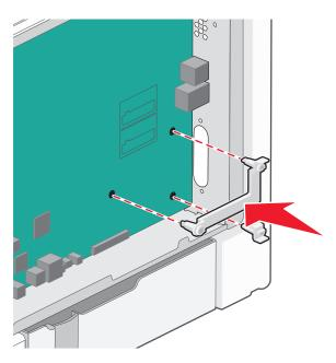
**6** Install the ISP on the plastic tee. Angle the ISP over the plastic tee, and approach the plastic tee so that any overhanging connectors will pass through the ISP opening in the system board cage.
