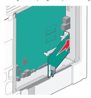
7 Lower the ISP toward the plastic tee until the ISP is seated between the guides of the plastic tee.
