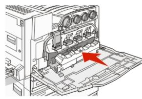
**10** Place the new printhead lens cleaner in the notches of Door E.
