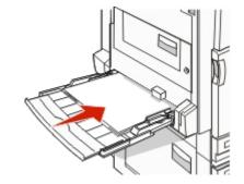
• Load A3, A5, B4, folio, legal, and statement paper with the recommended print side facedown and the short edge of the paper entering the printer first.
