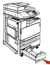
**2** Squeeze the length guide tab inward as shown, and slide the guide to the correct position for the paper size being loaded.
