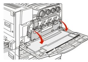
**4** Remove the old printhead lens cleaner from Door E, and then discard it.
