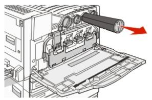
**6** Align the arrow-shaped handle with the unlock symbol, and then insert the toner cartridge all the way into the opening.
