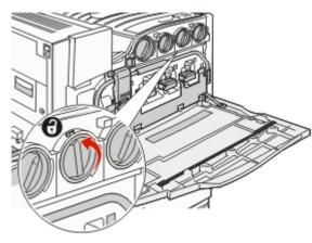
**5** Remove the cartridge by gently pulling it away from the printer.
