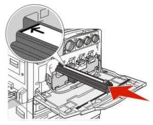
**6** Remove the tape from the top of the photoconductor.
