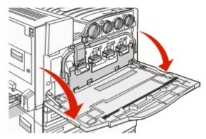
**Warning—Potential Damage:** To avoid overexposing the photoconductors, do not leave the door open for more than 10 minutes.
