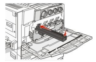
**8** Lift the bar up, and then press latch E5 down so that it holds the bar in position.
