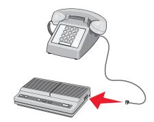
**5** Connect a third telephone cord from the answering machine to the EXT port of the printer.
