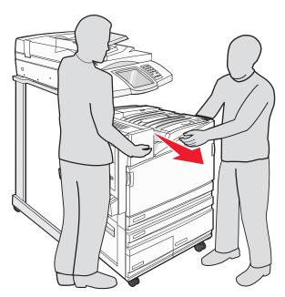
**CAUTION—TIPPING HAZARD:** If you need to roll the scanner and its shelf elsewhere, the scanner weighs 25 kg (55 lb); therefore, it requires two people to roll it safely.
