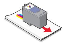
**4** Using another clean section of the cloth, gently hold the cloth against the contacts for about three seconds, and then wipe in the direction shown.
