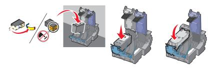
**Warning—Potential Damage:** Do *not* touch the gold contact area on the back or the metal nozzles on the bottom of the cartridge.
