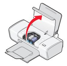
**3** Press down on the cartridge carrier lever to raise the cartridge carrier lid.
