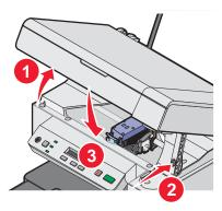
CAUTION: When closing the scanner unit, make sure to keep your hands out from underneath the scanner unit.
