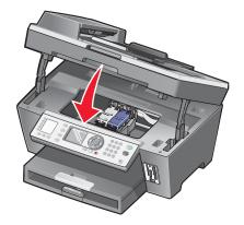
**Note:** The control panel display will prompt you to print an alignment page. For more information, see "Aligning print cartridges" on page 96.
