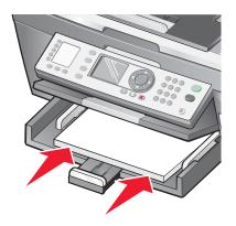
4 Adjust the paper guides to rest against the left, right, and bottom edges of the paper.
