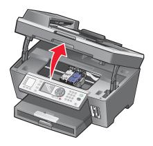
3 Press down on the lever to raise the cartridge lid.
